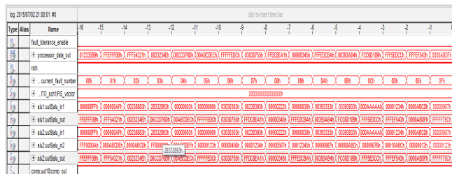
Fig: SignalTap FPGA emulation results without Faults
