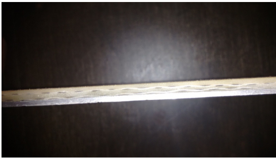
Fig 3.22 Cross sectional view of aluminium with FRP material
