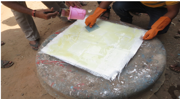
Fig : Woven roving bonding unidirectionally
