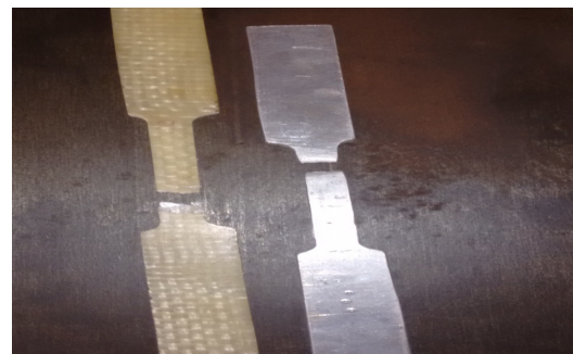
Fig Tensile specimens after test failure .
