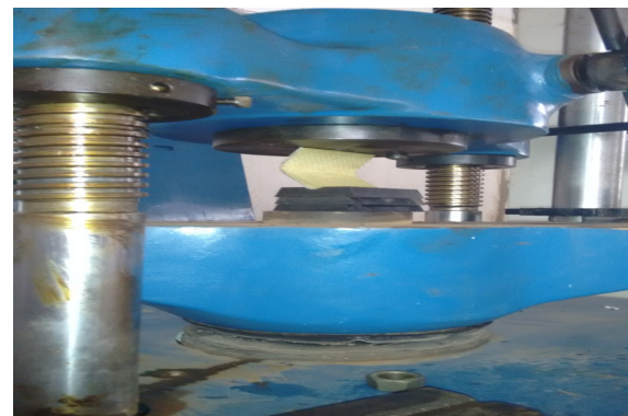
Fig: Compression test on UTM
