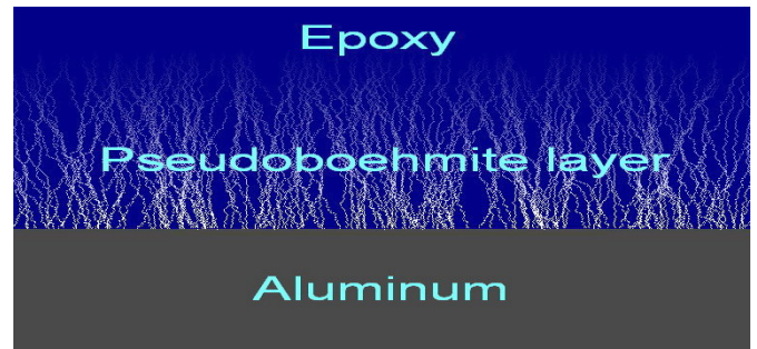
Fig. Schematic of formation of pseudoboehmiteoxy-hydroxide whiskers by immersion of Aluminum in boiling water.
