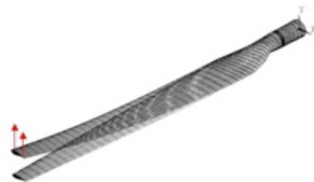
Figure 24. Application of a 500 lb flapwise tip load
