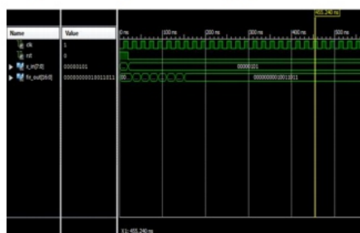
Fig. 14 Simulation output of FIR Filter using Improved CSLA
