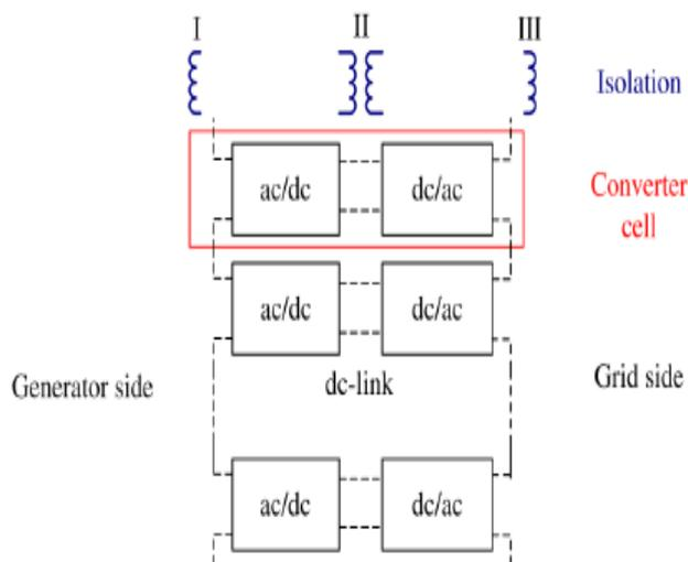
Fig. 1. Generalized cascaded multilevel converter topology (one phase leg).
