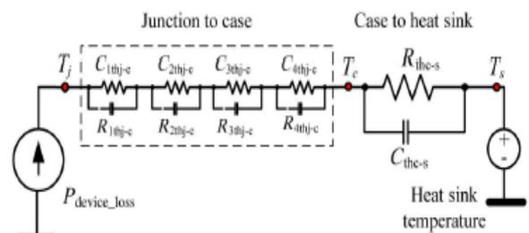
Fig.10. Thermal network to evaluate the device junction temperature.
