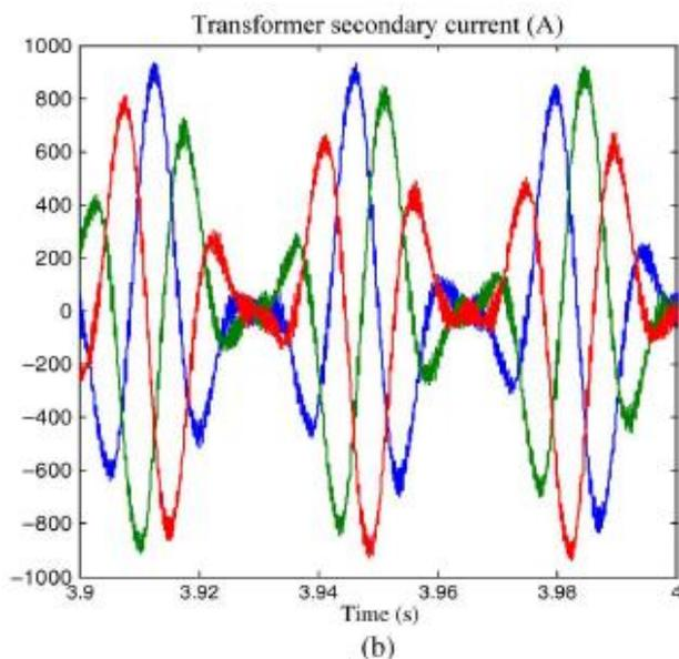
Fig.9. Inverter (transformer secondary) current with and without resonant controller applied: (a) without resonant controller and (b) with resonant controller.
