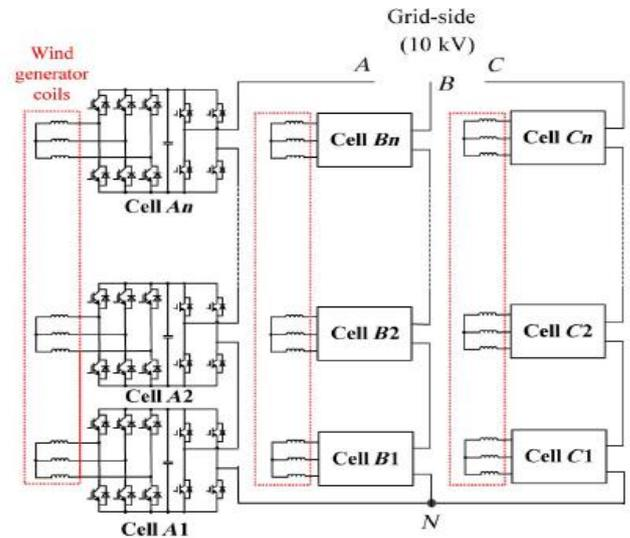
Fig.2. High-power, medium-voltage (10 kV) modular wind converter with generator-side isolation (converter type I).
