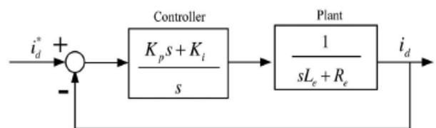
Fig.7. Current-loop diagram with a PI controller
