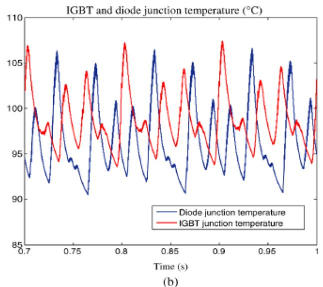
Fig.11. Inverter device (IGBT/diode) junction temperature variation: (a) without resonant controller and (b) with resonant controller.
