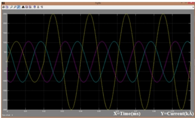
Fig.9 (b) Fault currents, during phase-to-ground downstream fault when DVR is inactive
