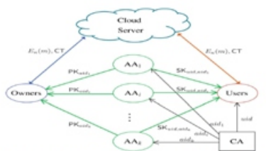
Fig. 1. System model of data access control in multi-authority cloud storage.
