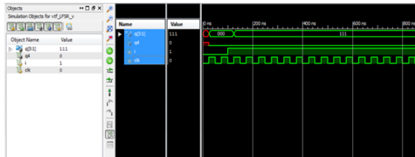
Fig 25. Simulation of pulse triggered reversible LFSR
