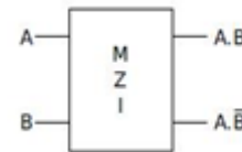
Fig. 1. Block diagram of Mach-Zehnder Interferometer switch [8]
