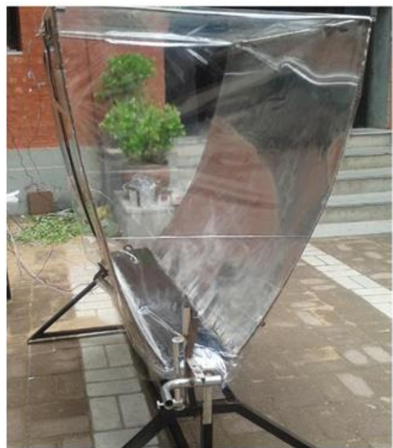
Fig 5. Compound Parabolic Concentrator
