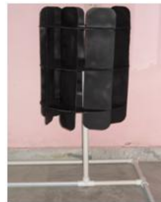
Fig. 17 Assembling of 8B VAWT Fig.
