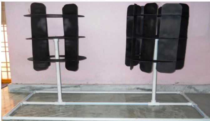
Fig. 19 Assembling of 4B & 8B VAWTS
