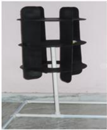
18 Assembling of 4B VAWT
