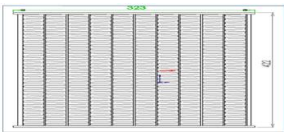
Figure 1: Radiator core model ( front view)
