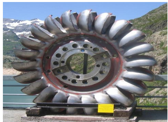
Fig 1.1 Pelton wheel impulse type water turbine
