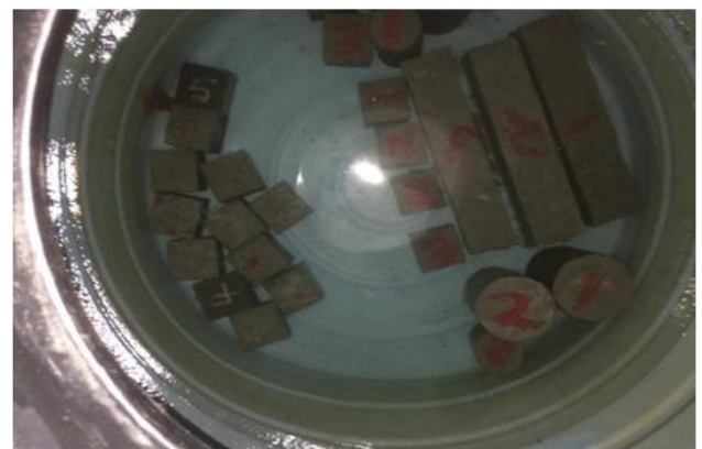
Fig 4.5: Curing of concrete specimens
