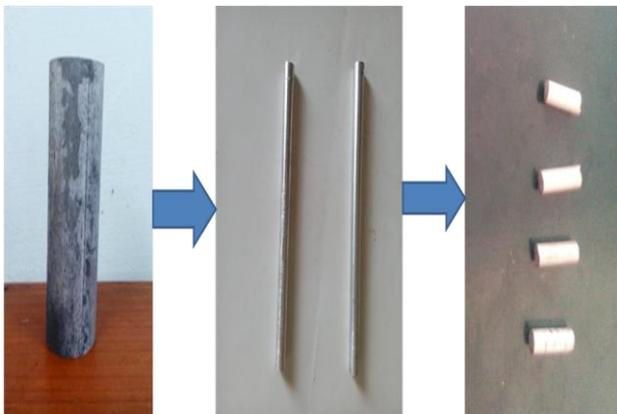
Fig. 1 Wear samples of AA 2024
