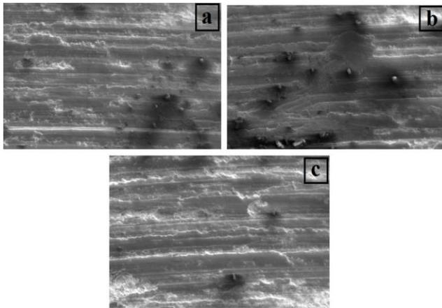
Fig 3 SEM micrograph wear track surface of AA 2024 alloy after T6 treated at 120°C for 20hrs in different conditions a) Cast b) Solutionized and c) Aged (120°C-20hrs) conditions
