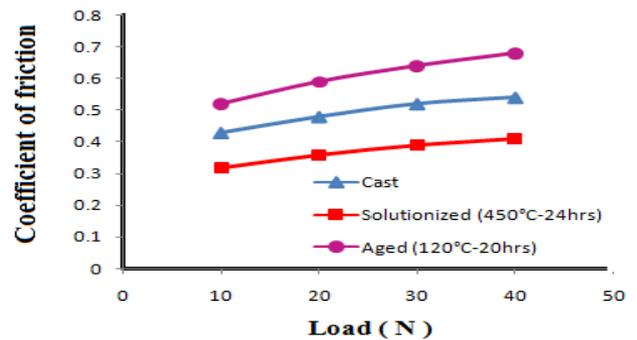
Fig 5 Coefficient of friction comparing different loads on AA 2024 alloy a) Cast b) Solutionized and c) Aged (120°C-20hrs)
