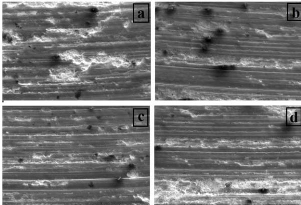
Fig 6 SEM micrograph wear track surface of AA 2024 alloy after T6 treated at 120°C for 20hrs in different conditions a) 10N, b) 20N, c) 30N and- d) 40N
