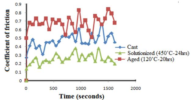
Fig 4 Coefficient of friction comparing time of wear on load at 40N, AA 2024 alloy a) Cast b) Solutionized and c) Aged (120°C-20hrs) conditions
