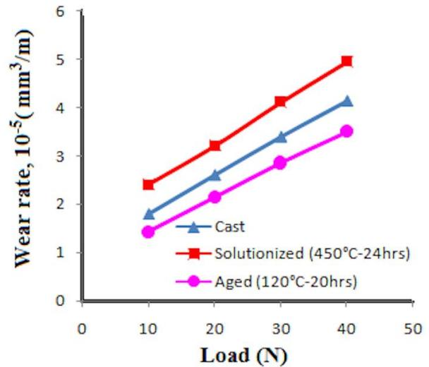
Fig. 2 Wear rate of different loads on AA 2024 alloy a) Cast b) Solutionized and c) Aged (120°C-20hrs) conditions
