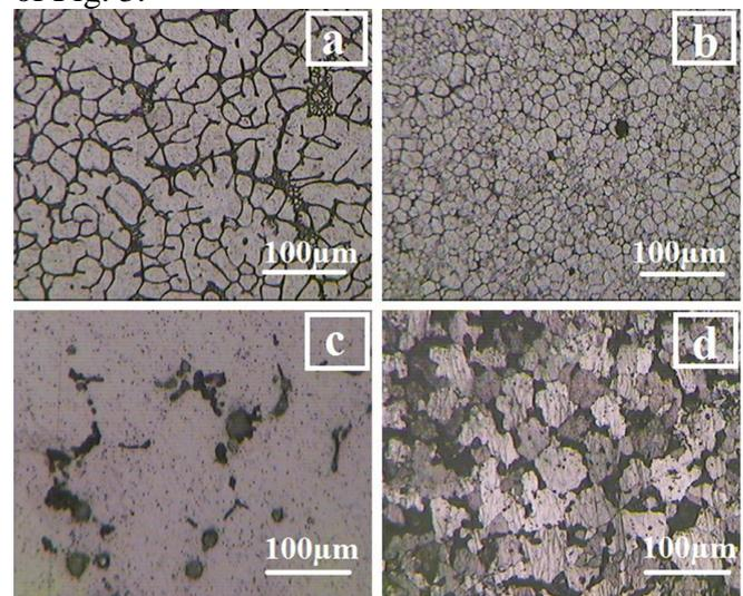
Fig. 2 Microstructure of AA7xxx alloy with different processing conditions (a) AA 7xxx Cast, (b) AA 7xxx + 1%Sc (b) AA 7xxx + 1%Sc Solutionized and (c) AA 7xxx + 1%Sc Aged.
