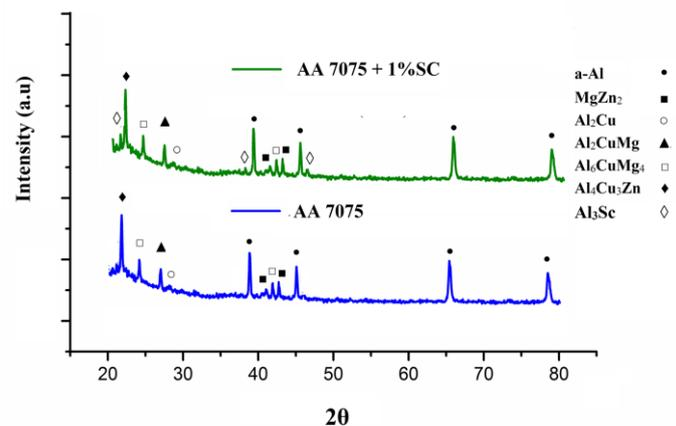
Fig. 3 X-ray diffraction patterns of AA 7xxx alloy and AA7xxx + 1%Sc
