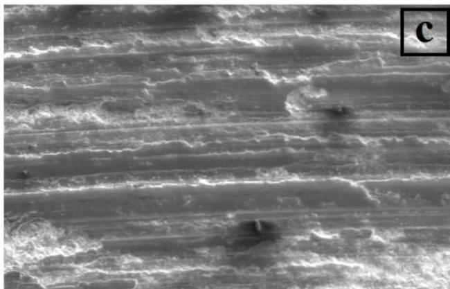
Fig 5 SEM micrograph wear track surface of AA 7xxx + 1%Sc alloy after T6 treated at 120°C for 20hrs in different conditions a) Cast b) Solutionized and c) Aged (120°C-20hrs) conditions
