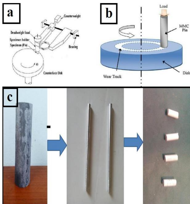
Fig1. a) Pin on disc set up b) Pin and disc contact c) Sample preparation from as cast.
