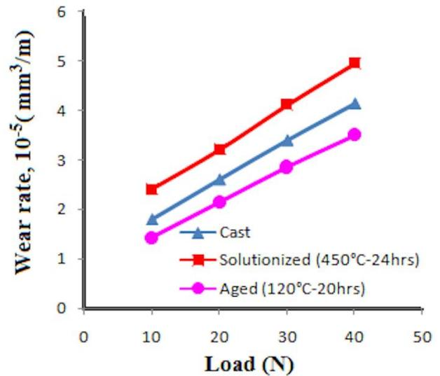
Fig 4 Wear rate of different loads on AA 7xxx + 1%Sc alloy a) Cast b) Solutionized and c) Aged (120°C-20hrs) conditions
