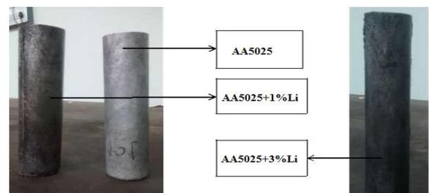
Fig. 1 Casting Billets of AA5025 Different Conditions
