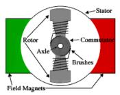
An electric motor is a machine which converts electrical energy into mechanical energy.
