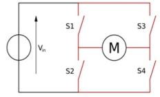
The two basic states of a H-bridge. The term "H-bridge" is derived from the typical graphical representation of such a circuit. An H-bridge is built with four switches (solid-state or mechanical). When the switches S1 and S4 (according to the first figure) are closed (and S2 and S3 are open) a positive voltage will be applied across the motor.
