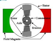
An electric motor is a machine which converts electrical energy into mechanical energy.
