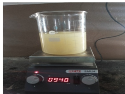
fig4: Separation of glycerol and bio fuel
