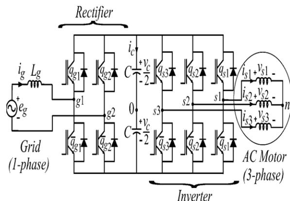
**Fig 1: Conventional 1-phase to 3-phase drive system.**
