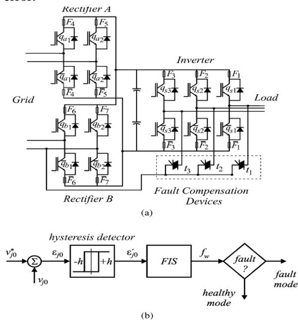
**Fig. 6: (a) proposed configuration highlighting devices of fault-tolerant system. (b) Block diagram of the fault diagnosis system.**
