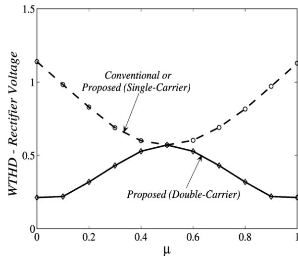
**Fig. 5: WTHD of rectifier voltage ( $v_{ab}$  for proposed configuration and  $v_g$  for standard configuration) as a function of  $\mu$ .**
