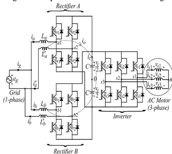
**Fig 2: Proposed single-phase to three-phase drive system with parallel converters.**
