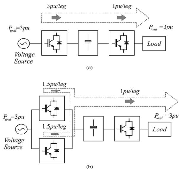
**Fig. 4: Flow of active power. (a) Conventional ac-dc single-phase to three-phase converter. (b) Proposed system with two rectifiers.**
