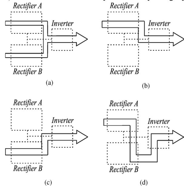
**Fig. 7: Possibilities of configurations in terms of fault occurrence. (a) Pre-fault system. (b) Post-fault system with fault at the rectifier B. (c) Post-fault system with fault at the rectifier A. (d) Post-fault system with fault at the inverter.**
