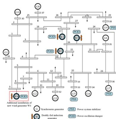
Fig. 2 Modified IEEE-39 bus New England system with DFIG wind turbines.
