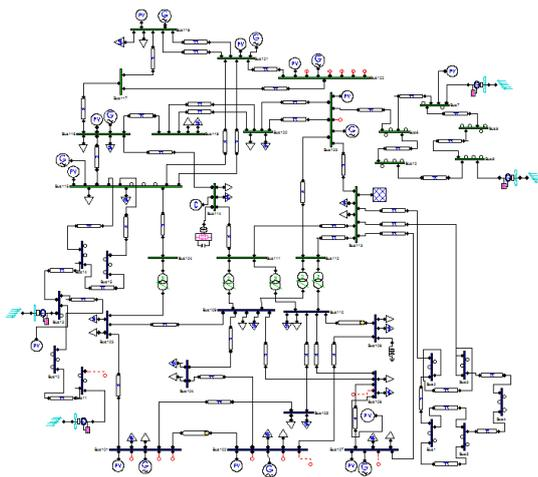
**Fig. 9 Simulation Circuit of IEEE-39 Bus System with STATCOM**
