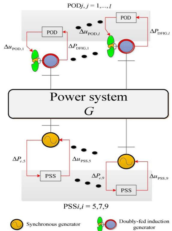
**Fig. 6 Power system with POD and PSS.**
