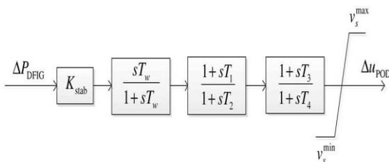
**Fig. 5 Structure of POD.**
