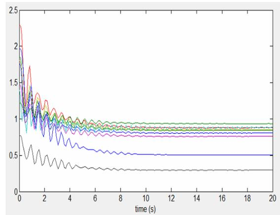
**Fig. 10 Generator Angles in Conventional System**
