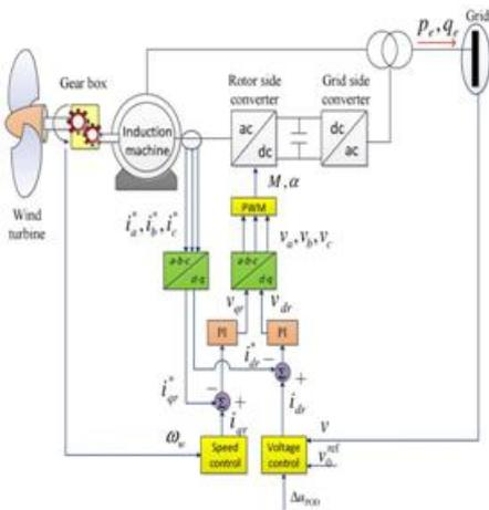
**Fig. 4 Configuration of DFIG wind turbine and control system.**
