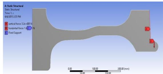
FIG: STRUCTURAL ANALYSIS- BOUNDARY CONDITIONS
