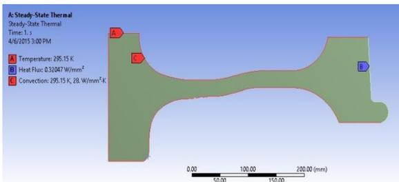
Fig Thermal analysis- boundary conditions
