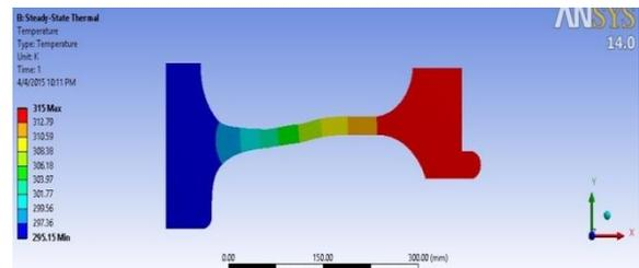
Temperature distribution under thermal load
