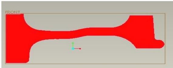
**FIG: MODIFIED DESIGN OF THE LOCOMOTIVE WHEEL CROSS- SECTION**
