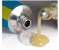
The applications For epoxy-based materials are extensive and include coatings, adhesives and composite materials such as those using carbon fiber and fiberglass reinforcements (although polyester, vinyl ester, and other thermosetting resins are also used for glass- reinforced plastic.
