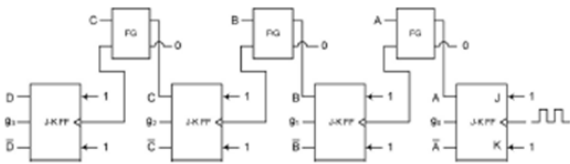
Fig. 5. Proposed design of 4-bit reversible sequence counter.
