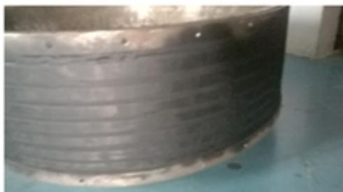
**Fig. 3. Flexible joint after Extraction**
