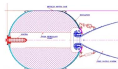
**Fig. 1. Propulsion system of a typical air borne vehicle**
