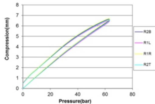
**Fig. 7. Seal Compression during Proof Pressure Test**
