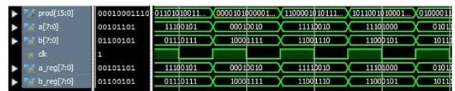
Figure 4. Simulation Result Of 16x16 Bit Vedic Multiplier
