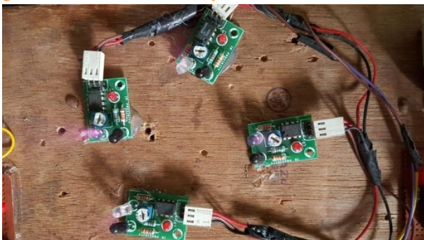
Fig. 12 IR sensors used for blind spot detection
