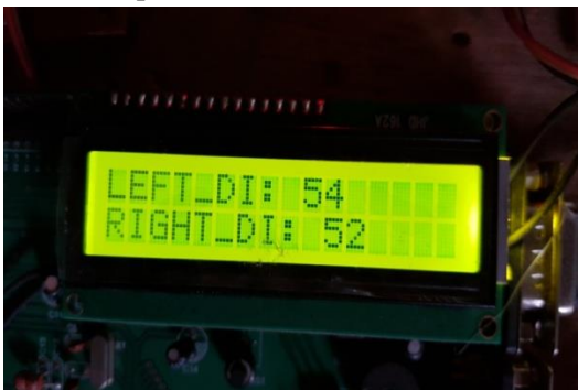
Fig.11 Distance measured by ultra sonic sensors
