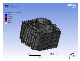
LOADS: Temperature -558 K Film Coefficient – 25 w/m<sup>2</sup> K Bulk Temperature – 313 K
