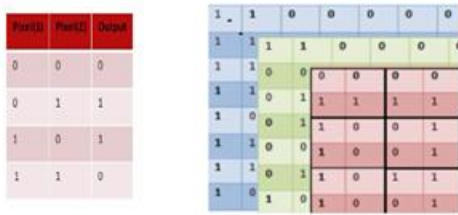
Fig. 5. EX-OR operation for detection.
