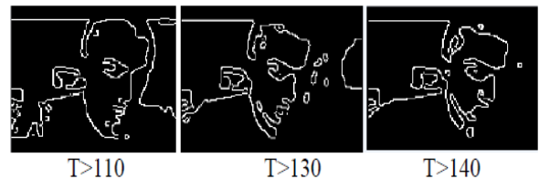
Fig. 3. Detection using canny detector at different threshold.
