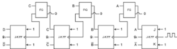
Fig. 5. Proposed design of 4-bit reversible sequence counter.
