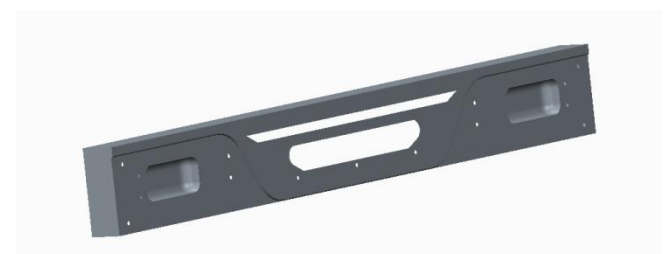
Fig.2 Geometric Model of the Steel bumper
