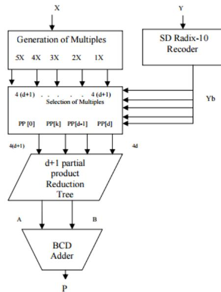
Figure:3 Combinational SD Radix-10 Architecture.
