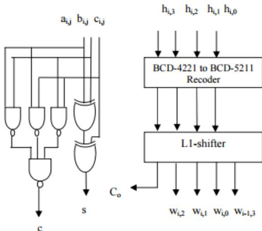
Figure: 2 Scheme of x2 for BCD-4221.
