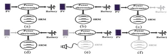
Fig. 3. Six operation modes of the proposed tri-port topology. (a) Mode 1. (b) Mode 2. (c) Mode 3. (d) Mode 4. (e) Mode 5. (f) Mode 6.
