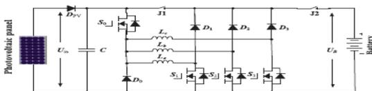
Fig. 2. Proposed tri-port topology for PV-powered SRM drive.
