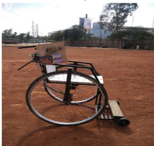
Figure (9) Voice operated intelligent wheelchair (Side view)
