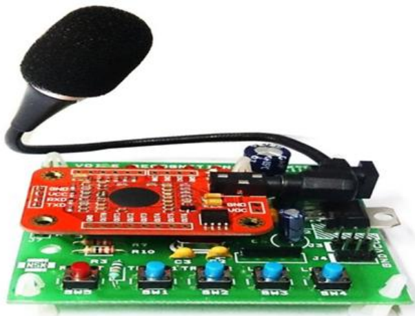
Figure(4) Voice Recognition Module (Arduino Compatible)
