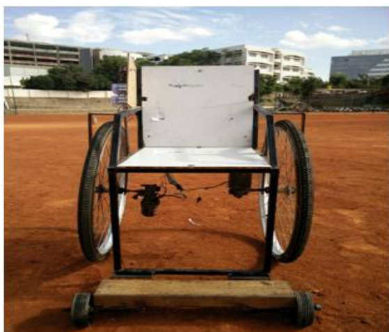
Figure (8) Voice operated intelligent wheelchair (Front view)
