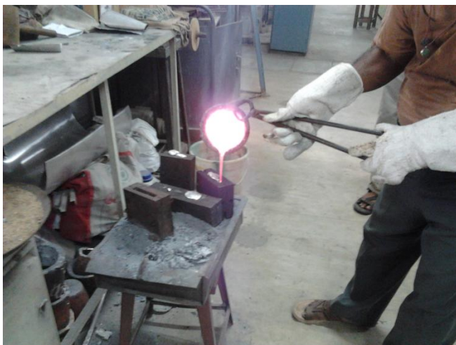
Figure3.4 Molten AAmatrix being casted
