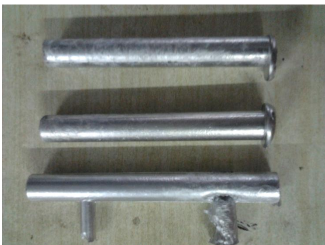
Figure3.5 Casted Aluminum rods
