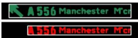
Fig. 16. Line detection in two passes, showing (top) detected text line after first pass and (bottom) detected text line after second pass.
