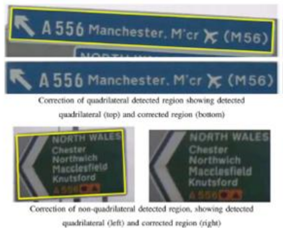
Fig. 14. Example detected regions with quadrilaterals and resulting corrected regions.
