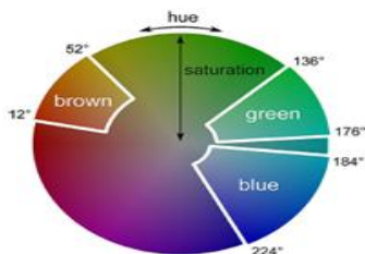
Fig. 7. Hue against saturation, with values for color traffic signs marked.
