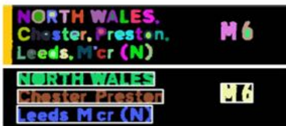
Fig. 15. Stages of line detection, showing (top) detected MSERs and (bottom) detected text lines.
