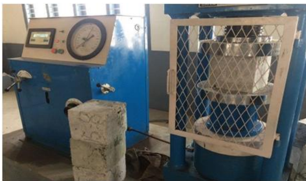
Cube placed in compressive testing machine
