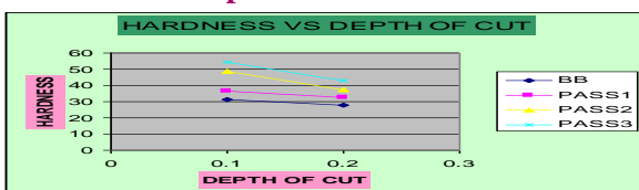
Fig 8.9 Variation of Surface Hardness with Depth of cut at Speed 14.13 m/min
