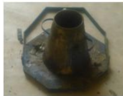
Fig.6.2 Slump cone apparatus
