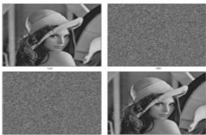
Fig. 4. (a) Original Lena, (b) Encrypted Lena, (c) Encrypted image containing embedded data with embedding size of 257 bits, and (d) Decrypted Lena.
