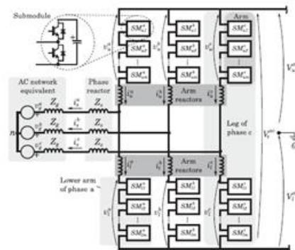
**Fig:2. Complete scheme of an MMC converter.**
