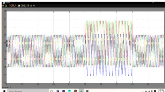
**Fig:6(m) capacitor MMC upper arm**
