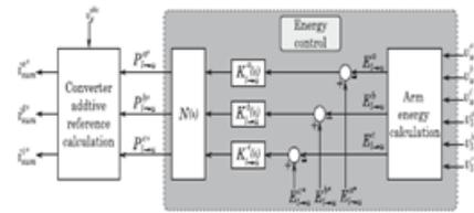
**Fig. 4. Upper-lower arms energy balancing control structure.**
