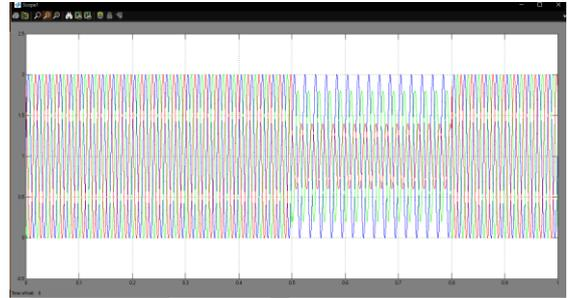
**Fig:8(b) MMC upper arm voltage**
