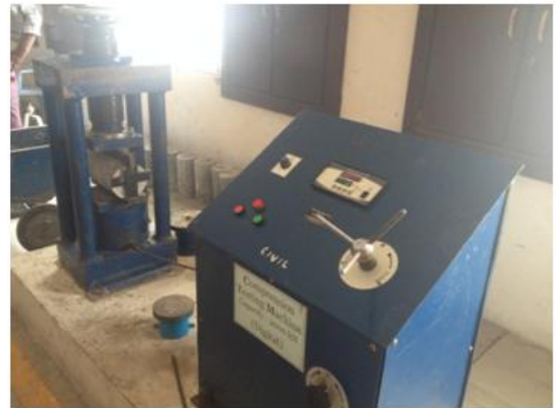
Fig 3.1.3 Split tensile set up in CTM
