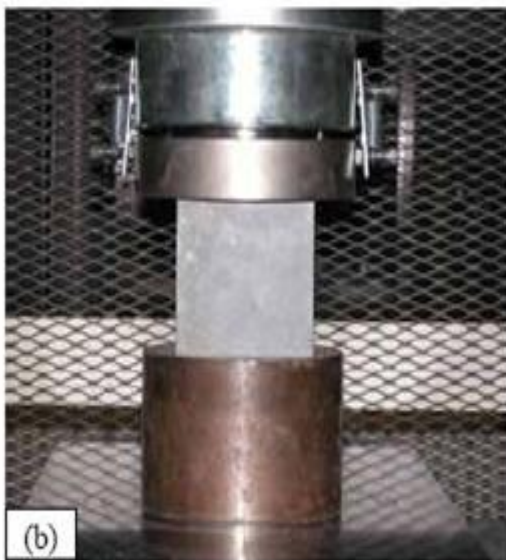
Fig No-4.2: Compressive strength testing machine
