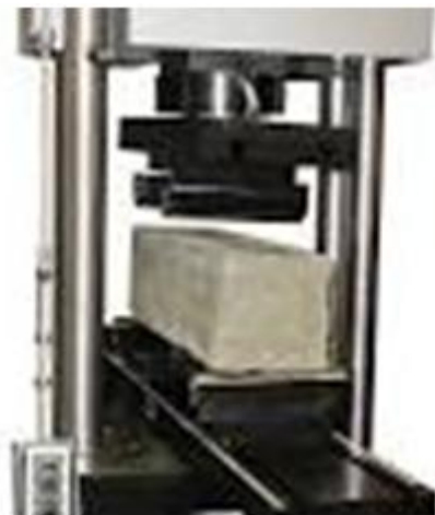
Fig 4.3: Flexural strength testing machine
