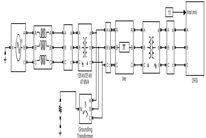
Fig 5: Simulation circuit of DFIG based WECS.
