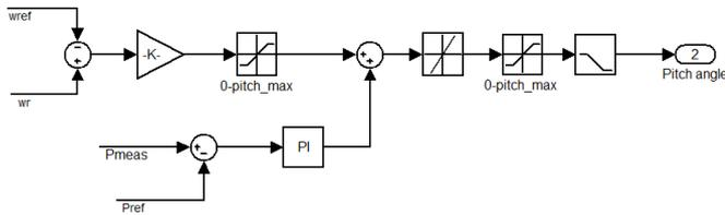
Fig 4: Pitch angle controller
