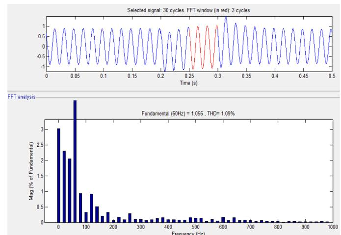
**Fig 13: FFT analysis of DFIG current between (0.25-0.3) sec (1.09%)**
