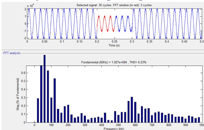
**Fig 13: FFT analysis of feeder voltage between (0.2-0.25) sec (6.23%)**
