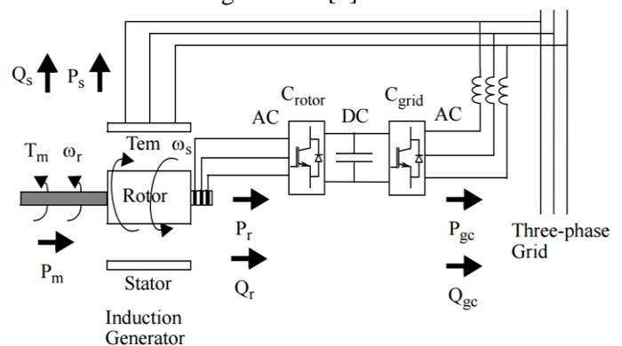
**Fig 1: The wind turbine and the DFIG system (Power Flow)**
