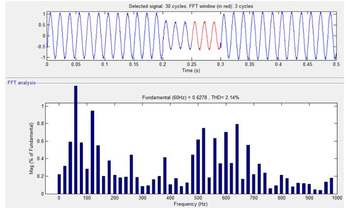
**Fig 11: FFT analysis of DFIG voltage between (0.25-0.3) sec (2.14%)**
