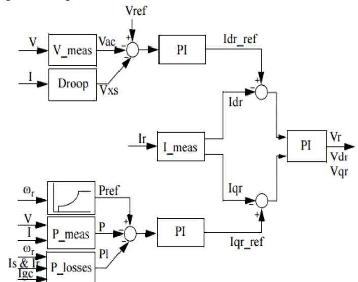
Fig 2: Rotor side converter control system
