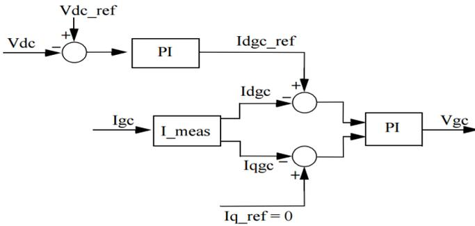
Fig 3: Grid side converter control system
