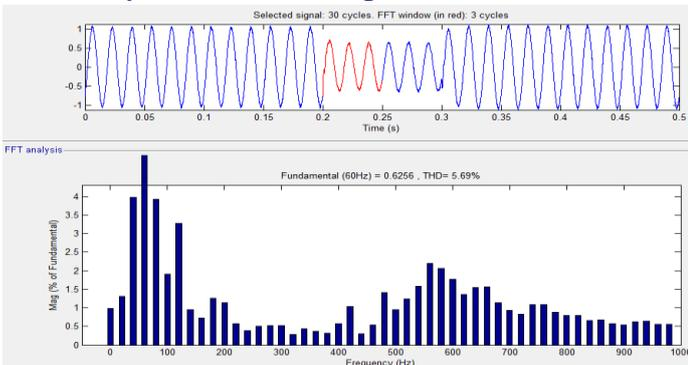
**Fig 10: FFT analysis of DFIG voltage between (0.2-0.25) sec (5.69%)**
