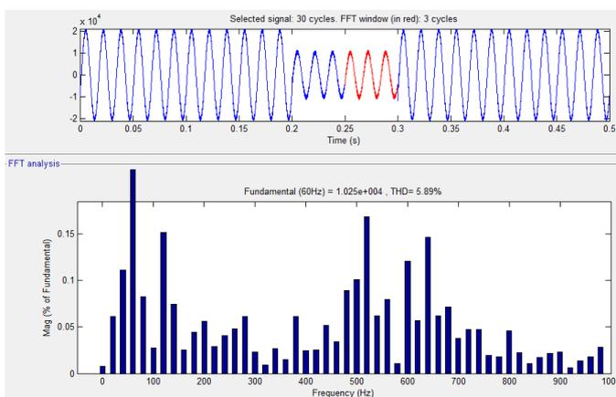
**Fig 13: FFT analysis of feeder voltage between (0.25-0.3) sec (5.89%)**
