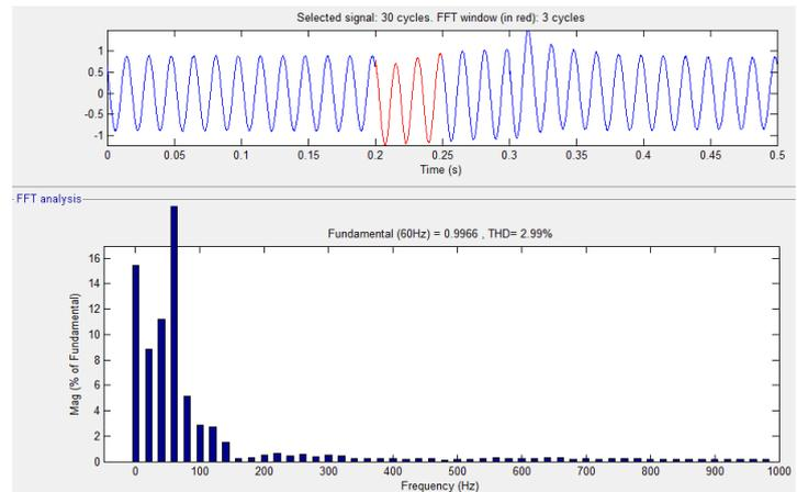
**Fig 12: FFT analysis of DFIG current between (0.2-0.25) sec (2.99%)**
