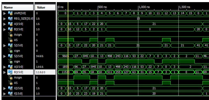
Figure 6: Waveform for rotation of coordinates with a given angle
