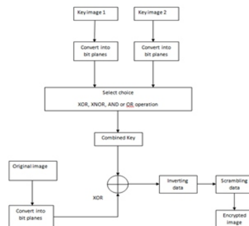
Fig.1 Proposed block diagram for Bitplane Crypt algorithm .
