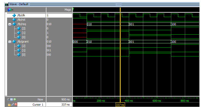
Figure 8: Simulation waveform of AHB Arbiter using Round robin Algorithm
