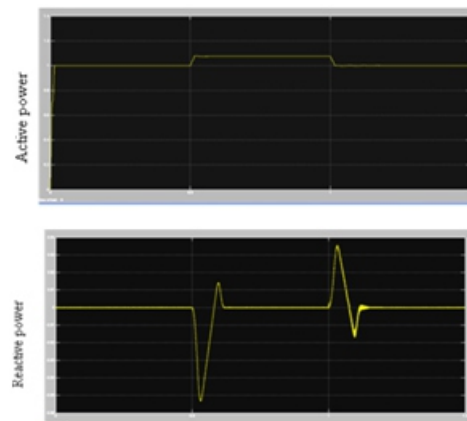
Fig.7 System response during load switching-inverter active & reactive power (load 1).
