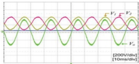
Fig 12. Output voltages of the boost inverter ( V_1 , V_2 , and V_o ) and dc input voltage, V_{in}
